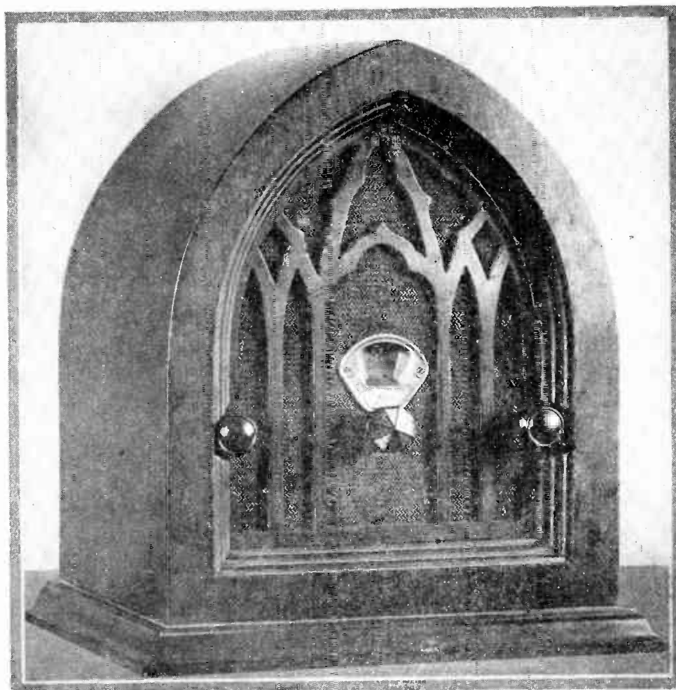
A Three Tube Pentode Midget Was Built Into a Cabinet That Formerly Housed Only a Speaker. See pages 6 and 7.
